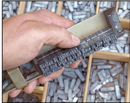
The small pieces of metal type, visible in the background in their typecase, are placed in a small metal tray called a composing stick. Lines of text are composed on the stick and then transferred to a metal frame called a printing form. The form is locked into the press, and pages are printed from it. After printing is complete, the type is removed from the form, cleaned, sorted, and returned to the typecase – ready for the next project.
